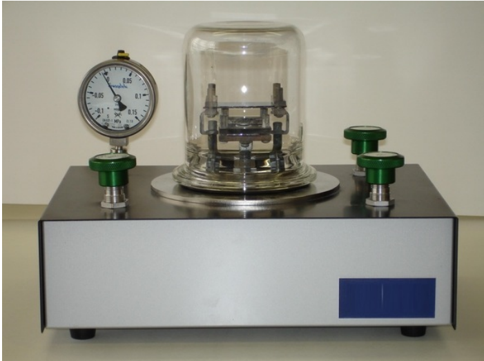
Simplified Creation Device of ZnO Nano Bar on Substrate]
