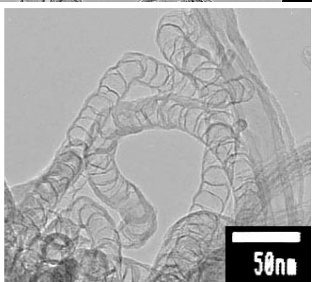
TEM Diagram of Hollow Tube-Shaped CNTs without N-Dope Treatment and Bamboo-Shaped CNTs after N-Dope Treatment
