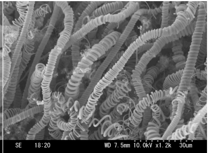
The Carbon Micro Coil created by the import of acetylene and co-catalyst
