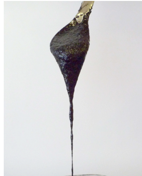
[CNTs/silicone paste of high viscosity and fluidity]
