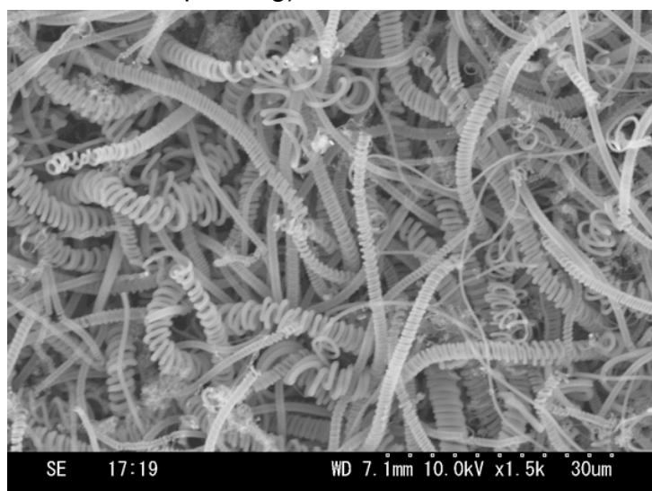
Carbon Nano-Coil made by ethyne and hydrogen SEM of CNTs Powders Created by Powder Carriers
